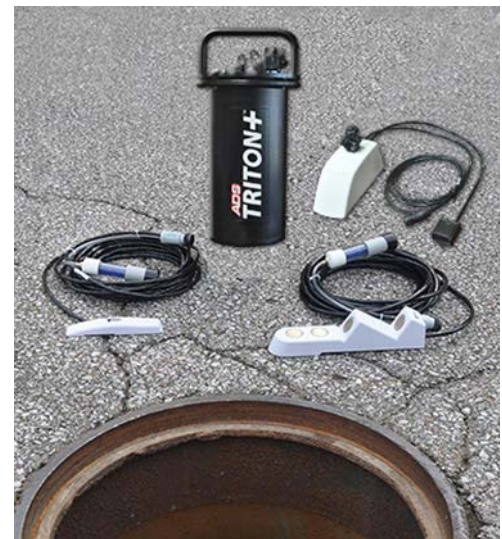
Figure 2.3 Triton Plus Meter and Sensors
